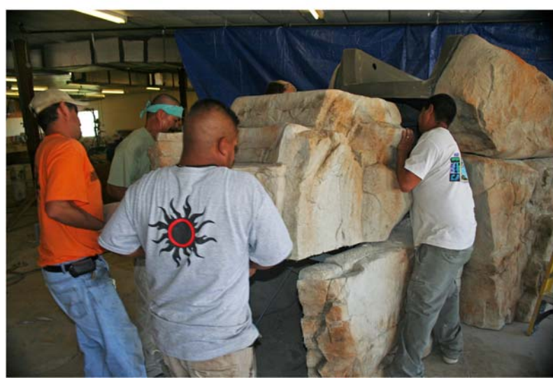
4. Set step frame and rock. Anchor wood rails to step assembly.
